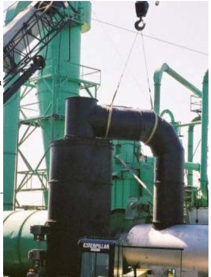
20 MM Btu/hr solid fuel burner for a drying system. Drying system retains capability of using natural gas as a fuel.
